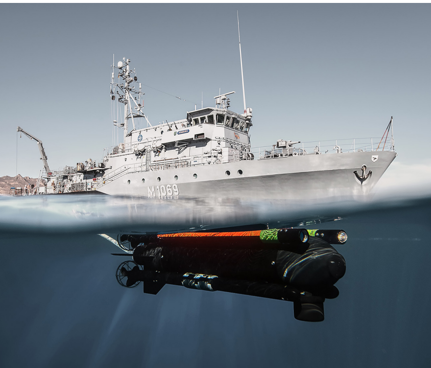
SeaFox® is a fibre-optic guided, one shot mine disposal vehicle
